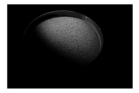
**MAKROPLUS® CC** are electroconductive concentrates based on thermoplastic matrix and highly electroconductive carbon black **CHEZACARB® AC**.
